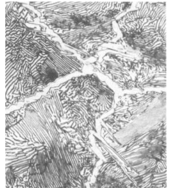
Atac chimic: Nital 3% x1000 Otel cu 1.4%C
