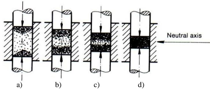
**FIG. 2.** Densification under double-acting effect of pressure
