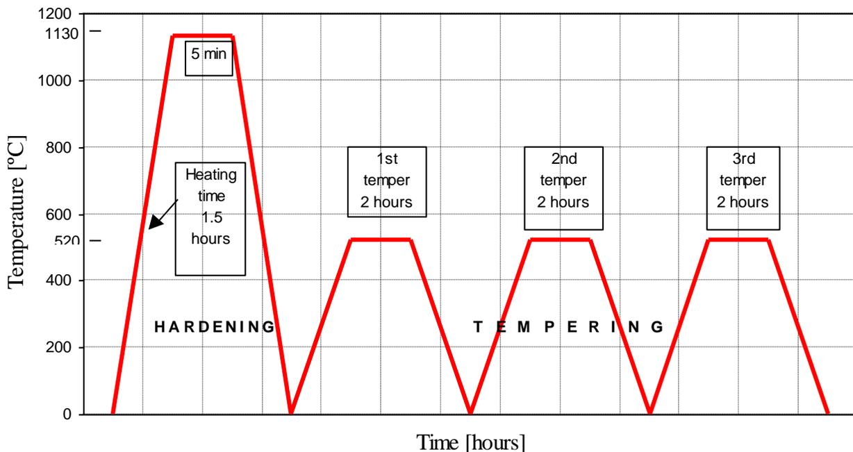
**Fig. 6** Cycles of heat treatment [2].
