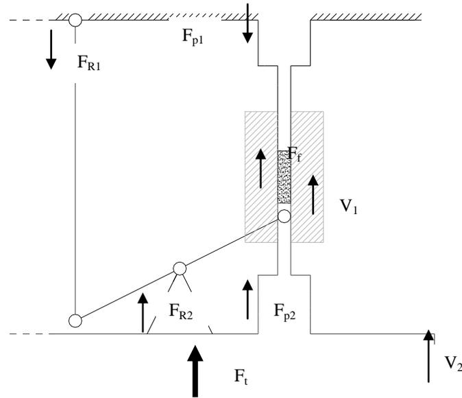
**Fig. 4.** Assisted friction compaction mechanism [2].
