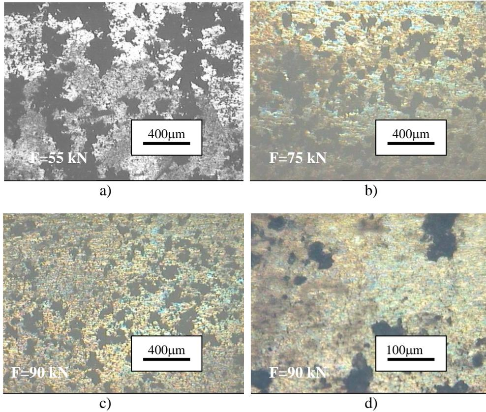
**Fig. 8.** Assisted friction compaction after sintering
