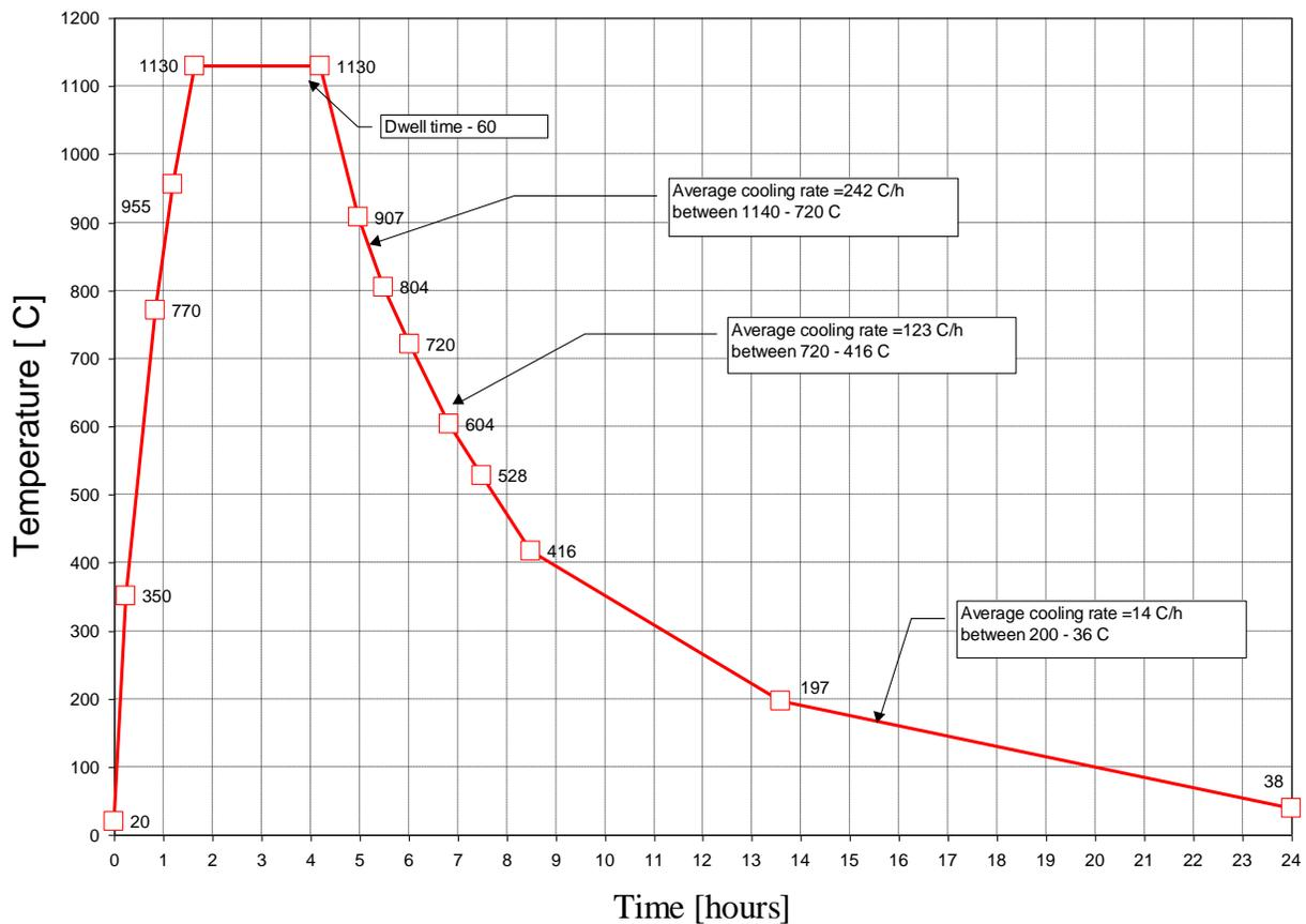
**Fig. 5.** Sintering diagram, at 1130<sup>0</sup>C [2].
