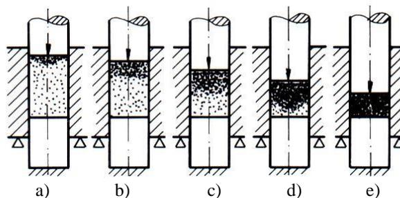
**Fig. 1.** -Densification under uniaxial effect of pressure.
