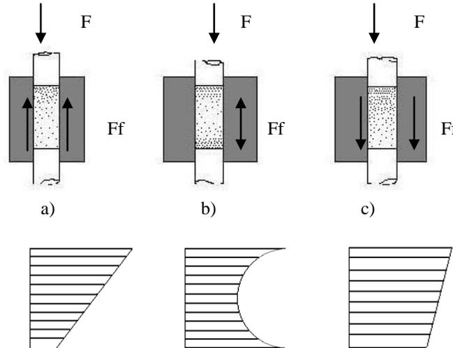
**Fig. 3.** Different methods of compacting and longitudinal profiles achieved
