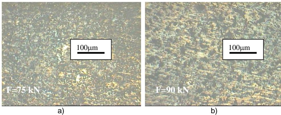
**Fig. 9.** Assisted friction compaction after heat treatment [2]
